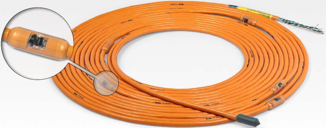
Model 3810 Thermistor String (inset shows a close-up of an encapsulated sensor).
