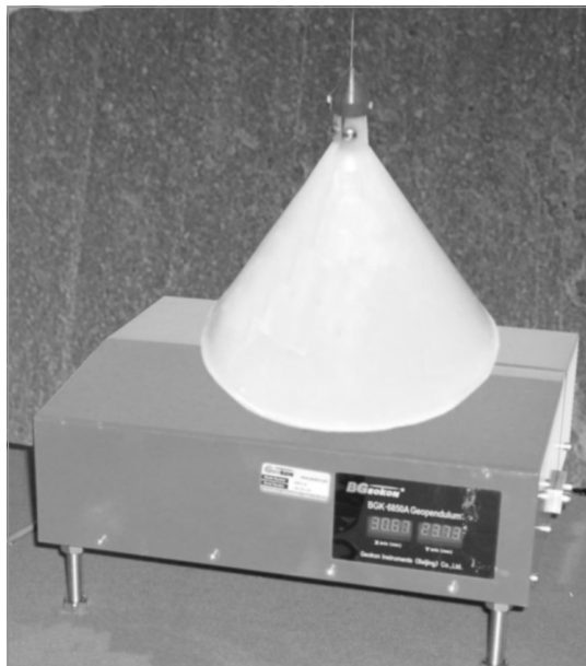
FIGURE 15: Conical Drip Shield Installed, with No Light Shield. Image for Reference Use Only
